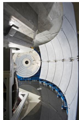
Head-high Si(111) analyzer crystals inside of the neutron backscattering instrument SHERES, FRM-II © Andreas Heddergott/ TU Munich
